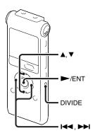
You can divide a message during playback, so that the message is divided into two parts and a new message number is added to the newer part of the divided message. By dividing a message, you can easily find the point from which you want to play back when you make a long recording such as at a meeting. You can divide a message until the total number of messages in the folder reaches the maximum number allowed.
